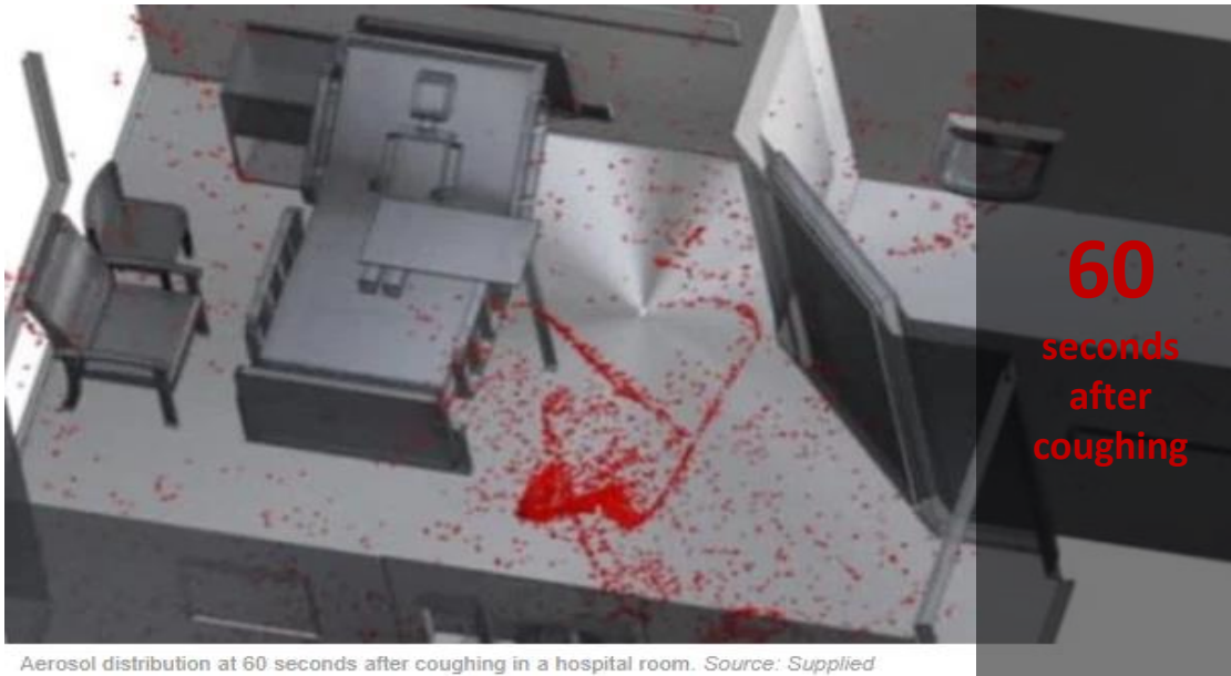
Aerosol distribution at 60 seconds after coughing in a hospital room. Source: Supplied
